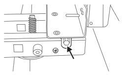
Make 10 complete (360°) turns clockwise. (This means turning and removing the levelling tool 20 times).
